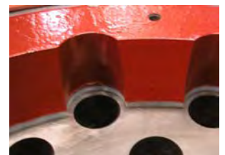
Taper Ring allows for fine adjustment of spacing between plates to control leak rate
