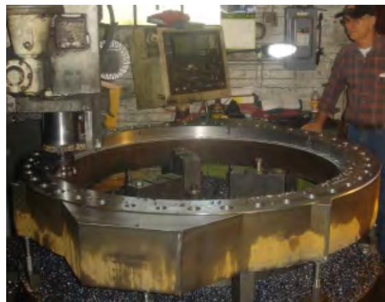
Available in sizes up to 90". 48" valve being manufactured in house by Ross Valve, shown above.
